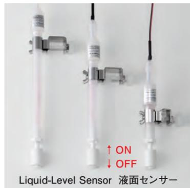
A type that automatically stops heating when the liquid level drops It is used in combination with a temperature controller and precision power supply. There are 3 stem sizes: L100mm (for 2~6inch tank), L170mm (for 8inch tank), L220mm.
