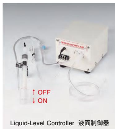
Liquid level controller with a liquid level sensor and a pump that replenishes water. When the liquid level drops, water is replenished to control the liquid level. Used alone (does not work with temperature controller)
